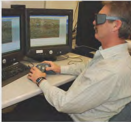
Figure 2. Digital, or softcopy, photogrammetric workstations support stereoscopic viewing and measuring in a 3D environment, where an overlapping pair of images is viewed with special polarized glasses.
